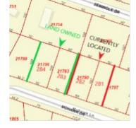
move forward with development. The field survey was conducted on lots 283 and 284 per the deed documents, yet the installation of utilities and the home moved forward on lots 281 and 282. (It appears that there was no construction survey for the actual house or utilities installations.) How do your field staff confirm they are
