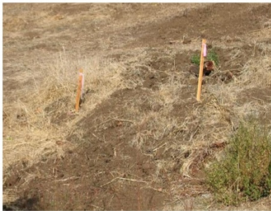
Surveyors often "flag" the corners when performing a field survey.
