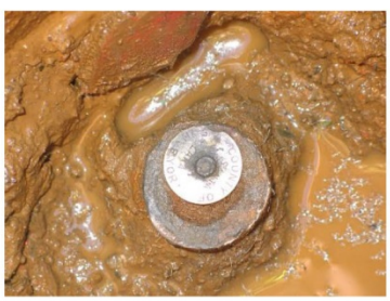
A brass tag with an LS number, RCE number or agency name typically is attached to the iron pipe. This identifies who set it.
