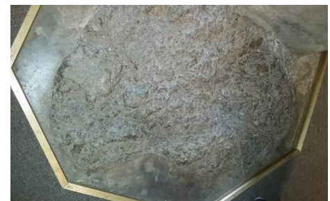
The peak of Mount Diablo, around which the Mount Diablo State Park Visitors’ Center was built. The depression in the rock is the actual “initial point” of all surveys in Nevada and most of northern California. (Photo courtesy of the author)
