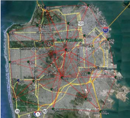
The 2013 regional network recovered the NAD83 (2011) & IGS08 (2005) datums based on 4 CORS: TIBB, P224, WINT and P176.
