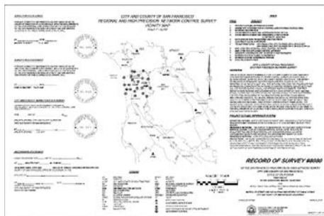
Survey results were published on a recorded map along with the new projection, CCSF-CS13, in early 2014.
