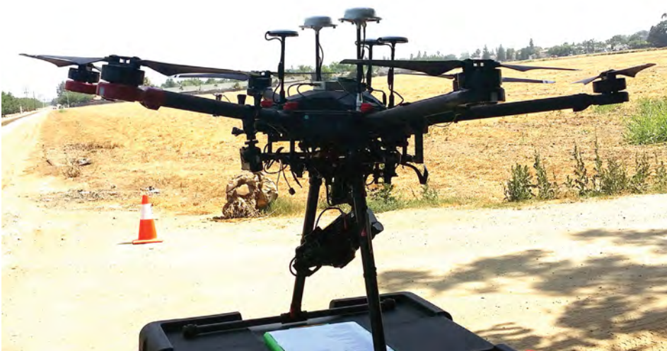
UAV – Matrice 600 Pro with RTK-GNSS positioning (photo by Jocelyn Correa)
