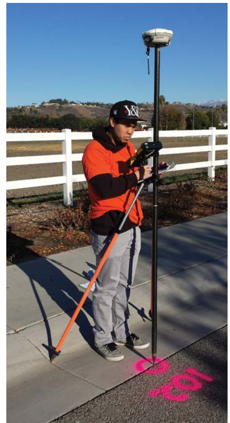
FIGURE 2: Rover system used for RTK and VRS data acquisition
