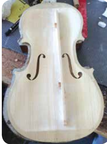
Chalk fitting a bass bar to the inside of the top. Tolerance-0 mm
