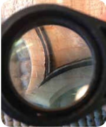
Inlaying purfling into the maple top. A channel 1.3 mm wide by 2 mm deep is hand cut around the parameter of the violin. Purfling is heat bent and fitted to the channel. This photo is through a magnifying glass to check the corner miter. The purfling is made from three sheets of veneer and cut into strips.
