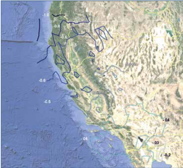
Figure 3: The contour map shows the difference in meters from derived heights using GEOID12A to xGEOID14B. This new geopotential datum, scheduled for implementation in 2022, is necessary to provide a height system commensurate with modern positioning capabilities, globally unified to address issues such as climate change and sea level rise.
