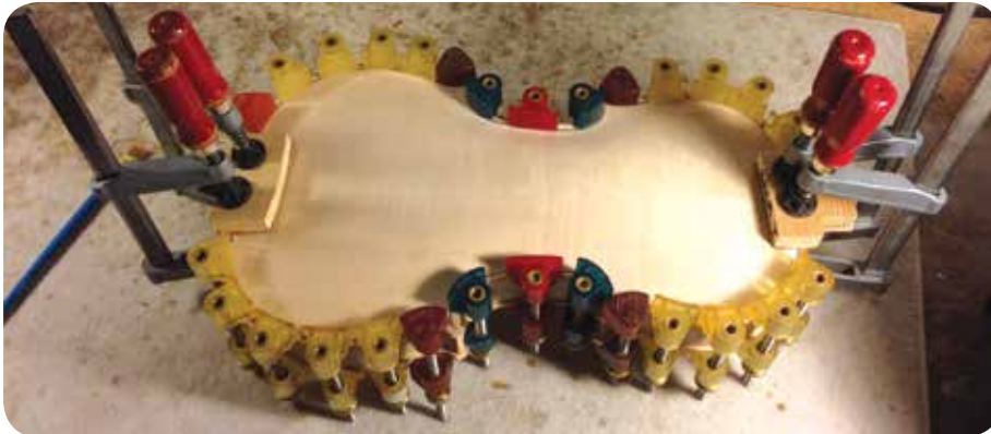
Ribs are 1 mm thick and heat bent to fit an inside mold. They are glued on to blocks. The mold is removed and the top and backs are glued to the ribs.
