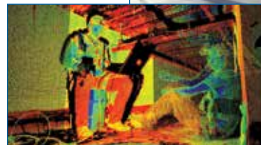
Static LiDAR captures high levels of detail with capability to map generally inaccessible areas and features. LiDAR processing includes identification and isolation of artifacts such as vehicles or people within the point cloud.
