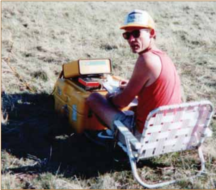
Dan Harrison, longtime County ROS map checker monitors a Trimble 4000 SST receiver during one of the 7 hour sessions
