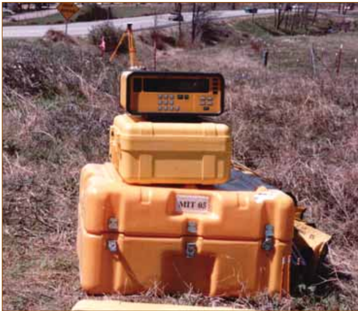
A Trimble 4000 SST GPS receiver borrowed from MIT at station SDGPS 15, a station set to replace the mark on Volcan Mountain which was inaccessible due to snow.
