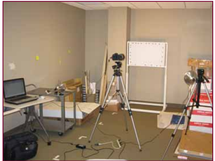
FIG. 1: The portable studio set up in the Shasta County Recorder's Office map room to shoot linen and blue print maps that couldn't be scanned.
