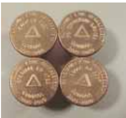
Special Monument caps for the retracement survey.
