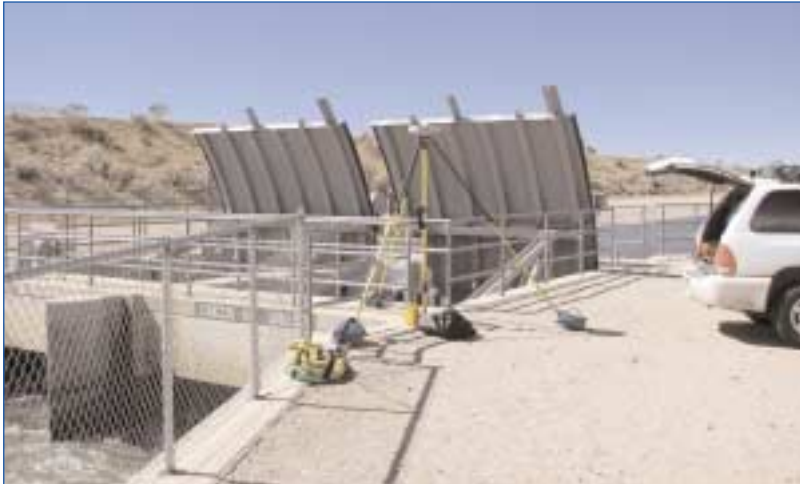
GPS Unit at Check 63. The Precise Surveys Unit performs a static survey along the East Branch of the California Aqueduct at a check structure. Benchmarks are located at all major structures and facilities along the State Water Project.
