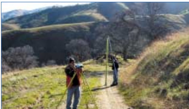
Precise leveling. Running first-order levels to the reference "rock mark" at Edmonston Pumping Plant are James Harlan (level) and Charles Mussett (rod).
