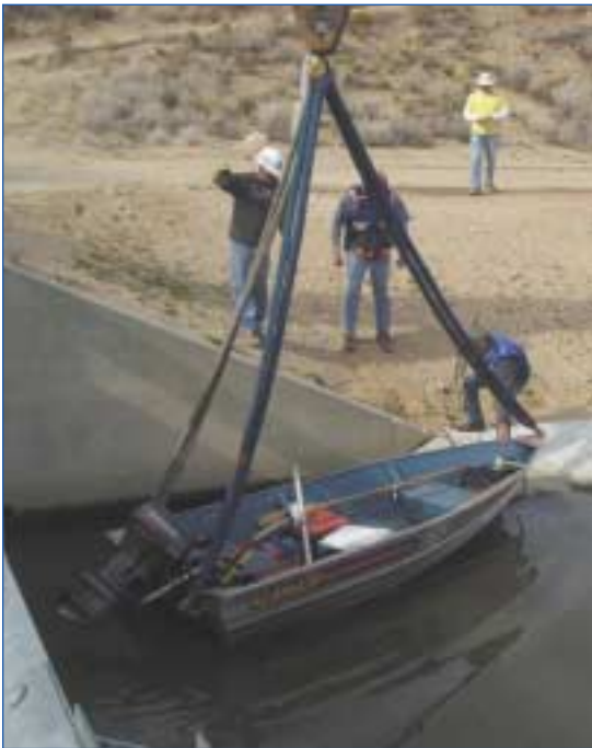
San Joaquin River bathymetry. Tim Johnston and Greg Sanfilippo of the Geodetic Branch collect bathymetry data to augment photogrammetric mapping for the San Joaquin River Restoration Program.
