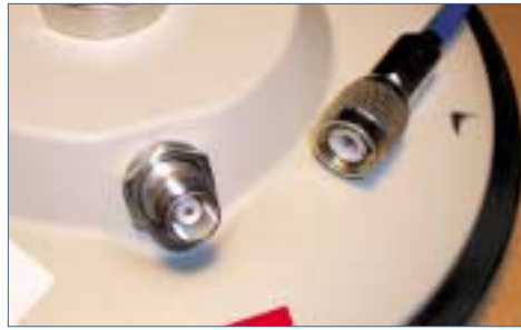
fig 2b – TNC female on left, TNC male on right (center post, internal threads).
