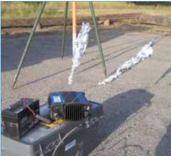
Fig 3a – Antenna model: Reynolds Oven Foil with Dry Cleaning hanger. Better for frat house TV than RTK data link.
