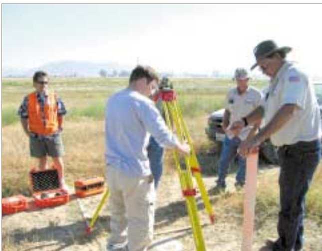
Setting up Tripod & Tribrach (Lt. to Rt. - Bill C., Ken J., Justin G., Ed K.)
