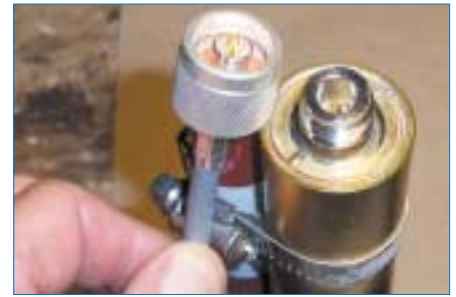
fig 2c – N-type male on left (center post, internal threads), N-type female on right.
