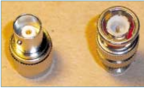
fig 2a – BNC female on left (posts on side of terminal), BNC male on right (center post, slots).
