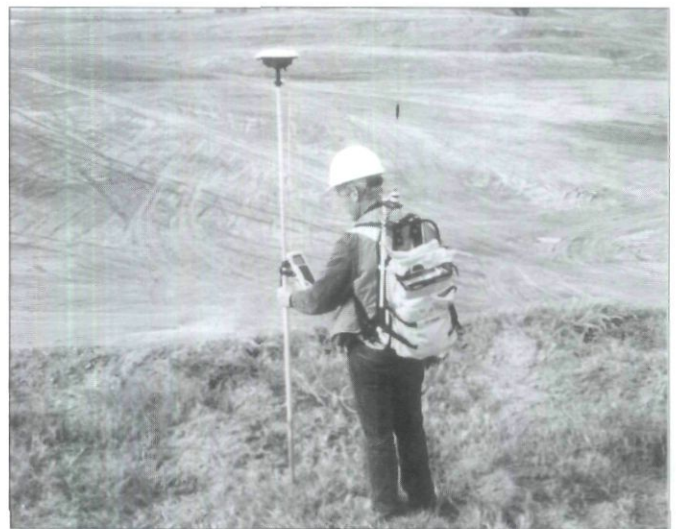
RTK Surveys to determine earth quantities
