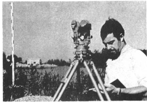
Subdivision surveying and layout using tacheometer.
