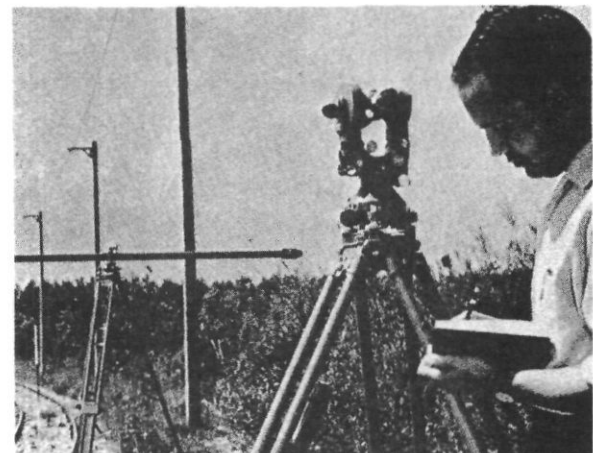
Distance measurement using subtense bar and theodolite.
