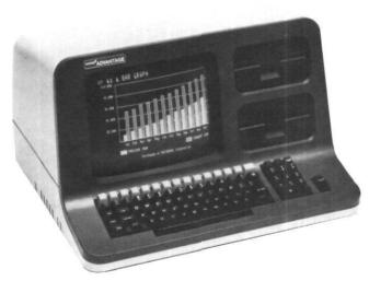
Basic system includes Northstar Advantage TM Computer with 64K RAM, IBM Selectric Keyboard, 640 x 240 bit mapped graphics, 2 360K disk drives, CPM® compatible Z-80 processor, green phosphor screen, serial port for printer, NS-100 132 column dot matrix printer, all survey software written in editable BASIC, startup supplies, business graphics package, diagnostic programs, 6 months warranty, complete documentation, a word processor, and screen plotting software.
