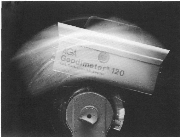
At touch of button, EDM itself displays accurate vertical angle reading
