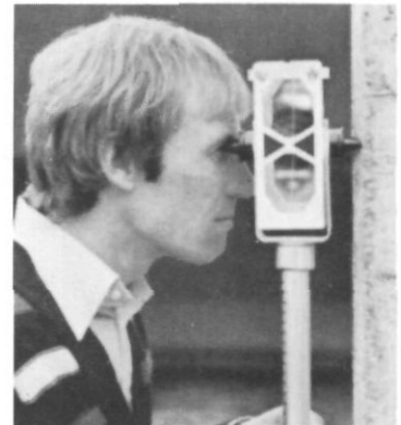
Reflector with target and right-angle prisms
