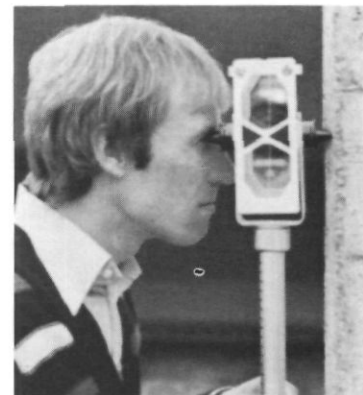
Reflector with target and right-angle prisms
