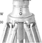
The Kern centering tripod is un matched in speed and simplicity of setup. (50 -250% faster for setups over point) Centering the bull's eye level on the centering rod not only centers the tripod but also automatically pre-levels the in strument support plate and gives the HI.
