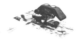
Instrument includes high-precision stereoscope, measuring system and drawing attachment. Used to measure elevations or to draw topographical details including contour lines directly from stereo aerial photographs.
