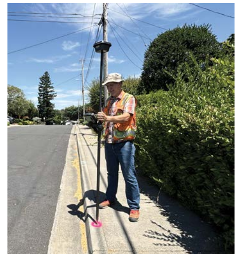
Collecting Tie Points the GPS Way.
