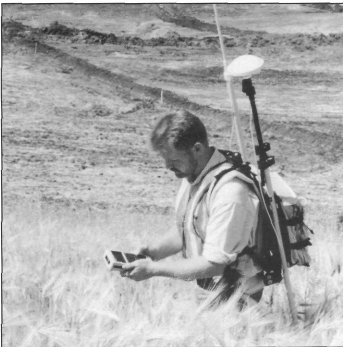
The Site Surveyor is a real-time, centimeter-level survey system for topographic, stakeout and control surveys. Using GPS and radio technology, it produces real-time output, so that surveyors simply walk to a point, and the measurement is known while observing the point
